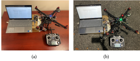
Figure 10: ConFIDE was evaluated in-lab on an S500 Pixhawk 2.4.8 UAV, propellers removed for safety. The setup included a UAV, radio controller, and a hardware Trojan for PWM inversion. Readings were processed via Arduino and Pymavlink
