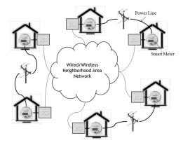
Fig. 1. The communication network between the smart meters.
