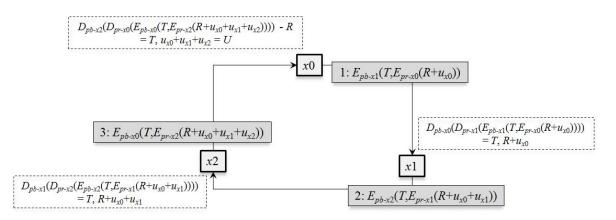
Fig. 4. The MPC technique for summing the usage vectors of the participating nodes that includes authentication and confidentiality security measures also.
