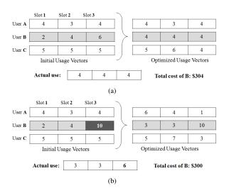
Fig. 6. Cost (price) of usage of a node (a) when it is truthful about its usage, (b) when it has lied about its usage (more than its actual requirement).
