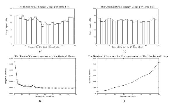
Fig. 7. (a) The initial total usage vector in different time slots (15 users), (b) the corresponding optimal total usage vector (after executing optimization process), (c) the energy cost (reduction) trend towards the optimal value with the number of iterations (rounds) of the optimization algorithm, and (d) the number of iterations that our proposed solution takes for convergence.
